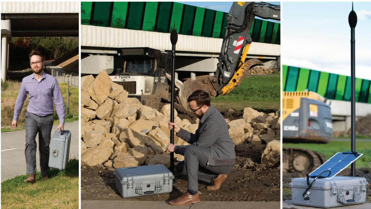
Confidently take unattended noise level measurements 24/7 with Noise Logger Type 3659. The reliable system enables you to cost-effectively:
