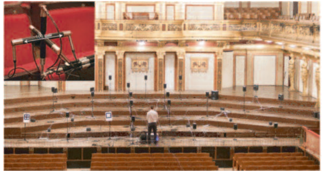
FIGURE 1: The loudspeaker orchestra on the stage of Musikverein, Vienna and the microphone array used to capture spatial impulse responses.
