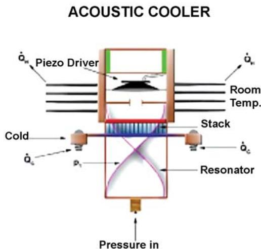
Figure 1 shows the acoustic driver coupled to a half-wave cylindrical resonator. The rate of heat extraction at the cold heat exchanger is  $Q_C$  and the rate of heat rejection at the hot heat exchanger is  $Q_H$ . The driver consists of a piezoelectric
