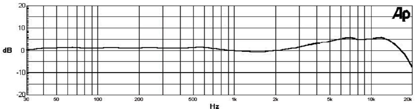
Fig. 4. Relative frequency response of the optical microphone.
